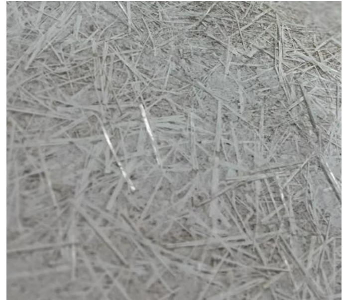
Typical GRC Mix – Spray Process
